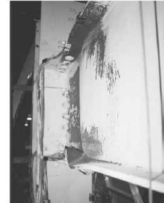
Figure 2-7. Web Local Buckling Limit State (SAC Project)
