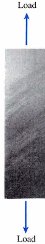
FIG. 2-38 Slip bands (or Lüders' bands) in a polished steel specimen loaded in tension
