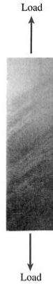
FIG. 2-38 Slip bands (or Lüders' bands) in a polished steel specimen loaded in tension
