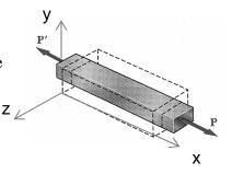
There exists a linear relationship while in the linear-elastic range of the material between *longitudinal strain* and *lateral strain*:
