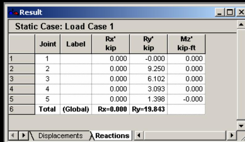
A screenshot of the 'Result' window titled 'Static Case: Load Case 1'. It displays a table of reaction values for joints 1 through 5, along with a total for the global system. The table has columns for Joint, Label, Rx' (kip), Ry' (kip), and Mz' (kip-ft). The 'Total (Global)' row shows Rx=0.000 and Ry=19.843. Below the table, there are tabs for 'Displacements' and 'Reactions', with 'Reactions' currently selected.
