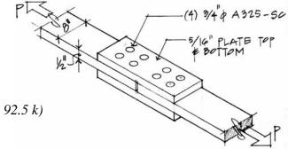
12B) Determine the capacity of the welded connection shown. The weld size is 3/16 in.. Assume the base metal is A36 steel and electrodes are E70XX in each problem. Use L = 4.5".
