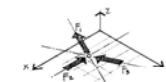
Coplanar, concurrent —All forces intersect at a common point and lie in the same plane. Figure 2.17(d) Particle or rigid body.
