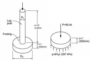
Using the following design values, determine the minimum size of D<sub>1</sub>
