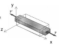
There exists a linear relationship while in the linear-elastic range of the material between *longitudinal strain* and *lateral strain*:
