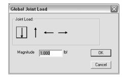
NOTE: Do not put support reactions as applied loads. The analysis will determine the reaction valuesMultiframe2D will automatically generate a grouping called a Load Case named Load Case 1 when a load is created. All additional loads will be added to this load case unless a new load case is defined (Add case under the Case menu).
