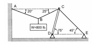
• CABLES: have the same tension all along the length if they are not cut. The force *magnitude* is the same everywhere in the cable *even if it changes angles*. Cables CANNOT be in **compression**. (They flex instead.)
