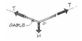
The shape of a cable having a *uniform distributed load* is almost parabolic, which means the geometry and cable length can be found with:
