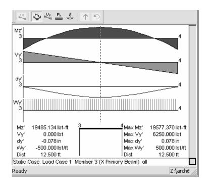
12. The Data window (D) allows you to view all data "entered" for the geometry, sections and loading. These values can be edited.
