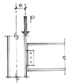
(a) Framed beam (shear) connection.
