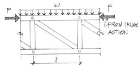
(d) Upper chord of a truss—compression plus bending.
