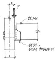
(c) Timber beam-column connection.
