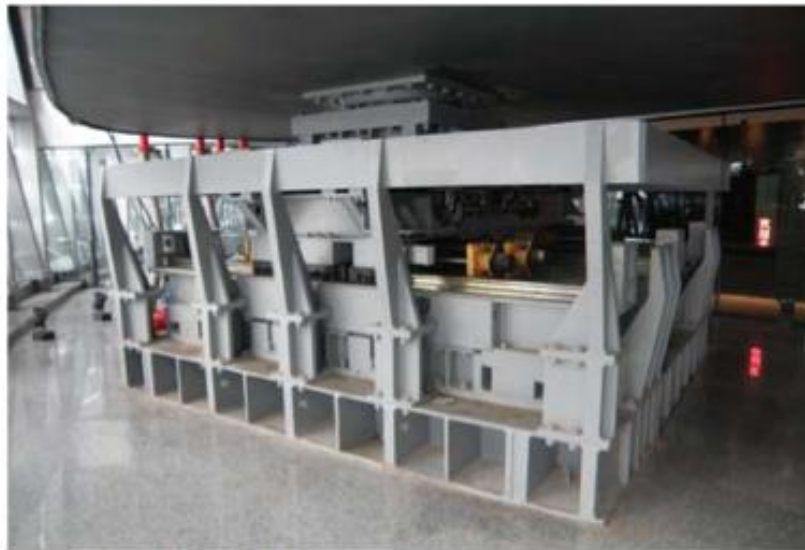
Figure 5. Bi-directional rail roller bearing © EERTC
