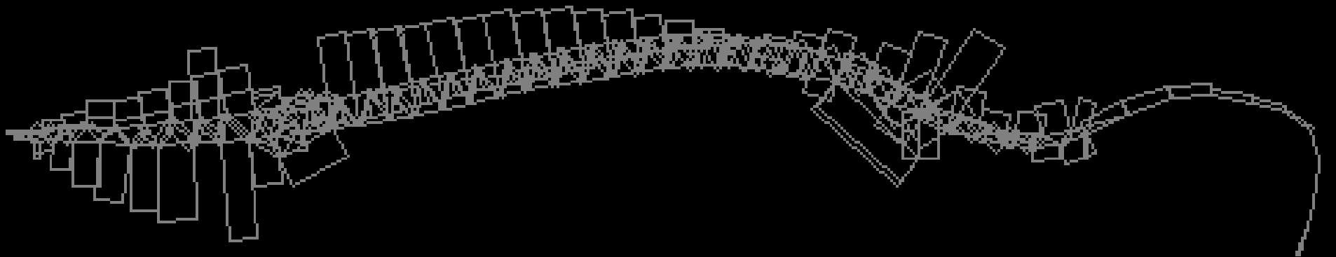
Exaggerated deformation under Lateral Loading
