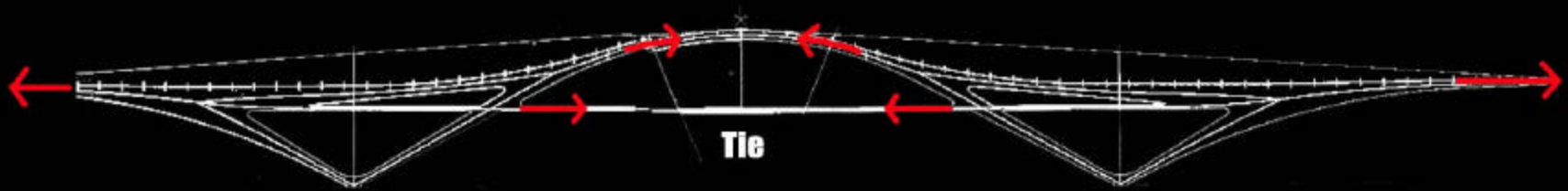
STRESS DISTRIBUTION THROUGH LONGITUDINAL SECTION
