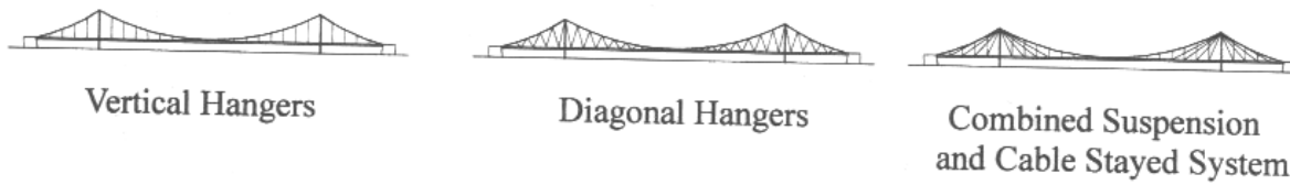
FIGURE 18.4 Types of suspenders.
