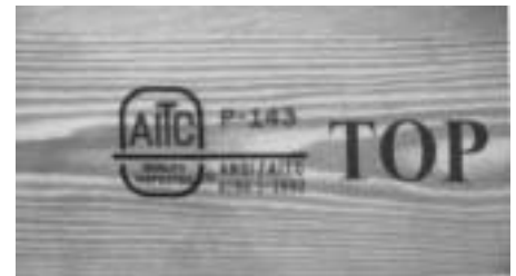
AITC mark of quality. The word "TOP" identifies beams with unbalanced sections.
