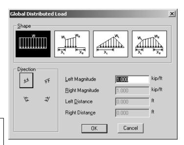
Multiframe4D will automatically generate a grouping called a Load Case named <u>Load Case 1</u> when a load is created. All additional loads will be added to this load case unless a new load case is defined (Add case under the Case menu).
