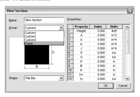
Table values 1-9 must have values for a Flat Bar, but not all are used for every analysis. A recommendation is to put the value of 1 for those properties you don't know or care about. Properties like  $t_f$ ,  $t_w$ , etc. refer to wide flange sections.
