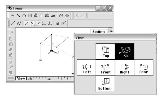
• If you wish to have additional beams supported by the beams of your frame, choose the beam and use the Subdivide Member menu under Geometry. This will make additional joints, but keep the segments together.
