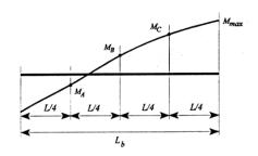
where C<sub>b</sub> is a modification factor for non-uniform moment diagrams where, when both ends of the beam segment are braced:
