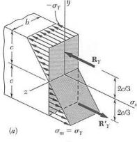
For a non-rectangular section and internal equilibrium at  $\sigma_y$ , the n.a. will not necessarily be at the centroid. The n.a. occurs where the  $A_{tension} = A_{compression}$ . The reactions occur at the centroids of the tension and compression areas.
