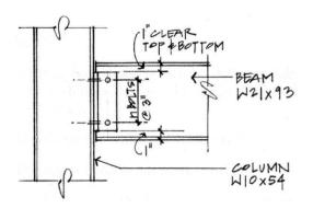
The maximum length the angles can be depends on how it fits between the top and bottom flange with some clearance allowed for the fillet to the flange, and getting an air wrench in to tighten the bolts. This example uses 1" of clearance:
