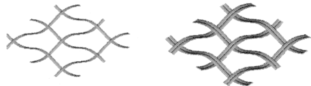
Fig. 1 Basket bond (left) and Panama bond
