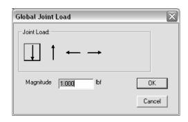
Multiframe2D will automatically generate a grouping called a Load Case named <u>Load Case 1</u> when a load is created. All additional loads will be added to this load case unless a new load case is defined (Add case under the Case menu).
