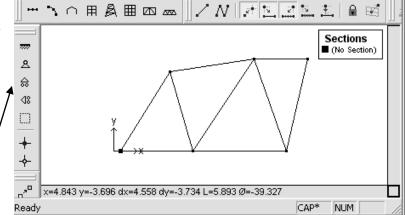
• The support types can be set by selecting the joint (drag) and using the Joint Toolbar (pin shown), or the Frame / Joint Restraint ... menu (right click).
