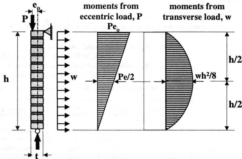
for large P and small w: critical location is at *top* of wall:  $M = Pe$
