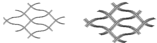
Fig. 1 Basket bond (left) and Panama bond
