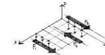
Noncoplanar, parallel—All forces are parallel to each other, but not all lie in the same plane. Figure 2.17(e) Rigid bodies.
