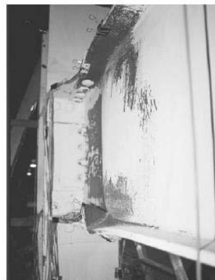
Figure 2-7. Web Local Buckling Limit State (NAC Project)
