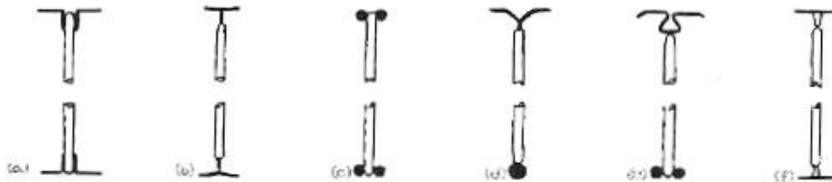
(c) SECTION THRU JOISTS SHOWING FLANGE TYPES
