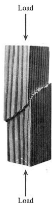
FIG. 2-37 Shear failure along a 45° plane of a wood block loaded in compression
