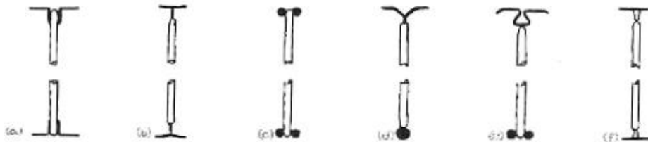
(c) SECTION THRU JOISTS SHOWING FLANGE TYPES
