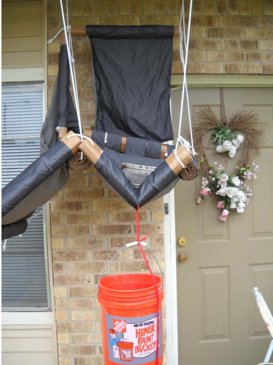
Figure 8: Testing for Bending Capacity
