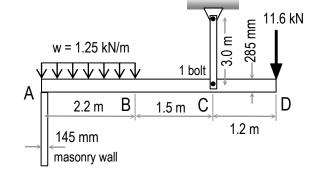
roller support) and with a metal strap and bolt at point C (considered a pin). The beam is loaded as shown.
