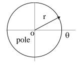
Definition: Radius of Gyration; the distance from the moment of inertia axis for an area at which the entire area could be considered as being concentrated at.
