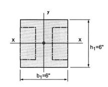
Determine the moments of inertia about the centroid of the shape.
