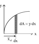
A shape that has area at a greater distance away from an axis through its centroid will have a **larger** value of I.
