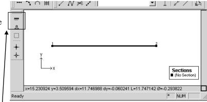
• The support types can be set by selecting the joint (drag) and using the Joint Too bar (pin shown), or the Frame / Joint Restraint ... menu (right click).
