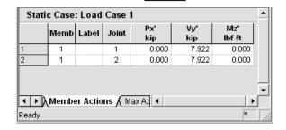
NOTE: Px' refers to the axial load (P) in the local axis x direction (x'). Vy' refers to the shear perpendicular to the local x axis, and Mz' refers to the bending moment.
