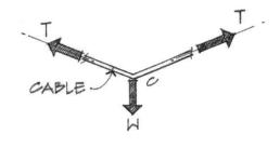
The shape of a cable having a *uniform distributed load* is almost parabolic, which means the geometry and cable length can be found with:
