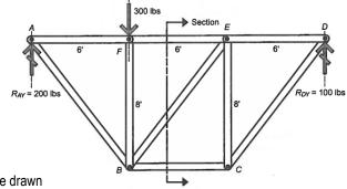
There can be only two intersections when two of the three forces are parallel – at E and B:
