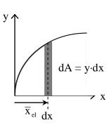
A shape that has area at a greater distance away from an axis through its centroid will have a **larger** value of I.
