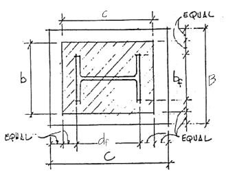
$b = b_f + \frac{(B - b_f)}{2}$  where  $b_f$  is the width of column flange and B is base plate side
