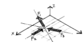
Coplanar, concurrent —All forces intersect at a common point and lie in the same plane. Figure 2.17(d) Particle or rigid body.
