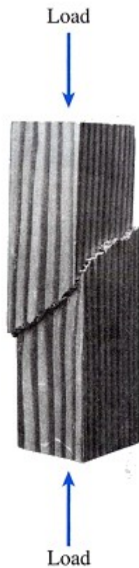
FIG. 2-37 Shear failure along a 45° plane of a wood block loaded in compression
