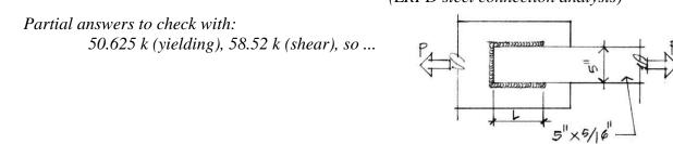
(15%) 11C) Determine the capacity and adequacy of the framed beam connection shown when the factored beam reaction is 300 k and ½" angles of sufficient length are used. The column and beam are A992 steel. The angles are A36 steel with 3" spacing of holes and 1 ¼" edge distances (*see table*). The bolts are A490-X. (*LRFD steel connection analysis*)
