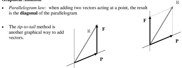
• With **3** (three) or more vectors, successive application of the parallelogram law will find the resultant *OR* drawing all the vectors **tip-to-tail** in any order will find the resultant.
