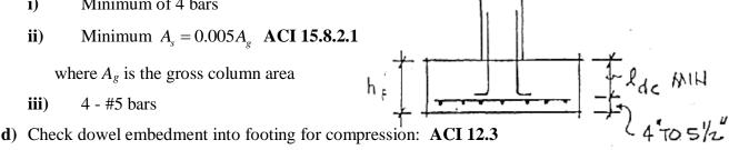
$l_{dc} = \frac{0.02 f_y d_b}{\sqrt{f'}}$  but not less than  $0.0003 f_y d_b$  or 8" where  $d_b$  is the bar diameter
