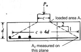
Req. dowel  $A_s = \frac{\phi P_{dowels}}{\phi f_{..}}$  where  $\phi = 0.65$  and  $f_y$  is the reinforcement grade
