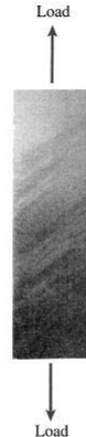
FIG. 2-38 Slip bands (or Lüders' bands) in a polished steel specimen loaded in tension
