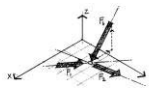
Noncoplanar, concurrent —All forces intersect at a common point but do not all lie in the same plane. Figure 2.17(f) Particle or rigid bodies.
