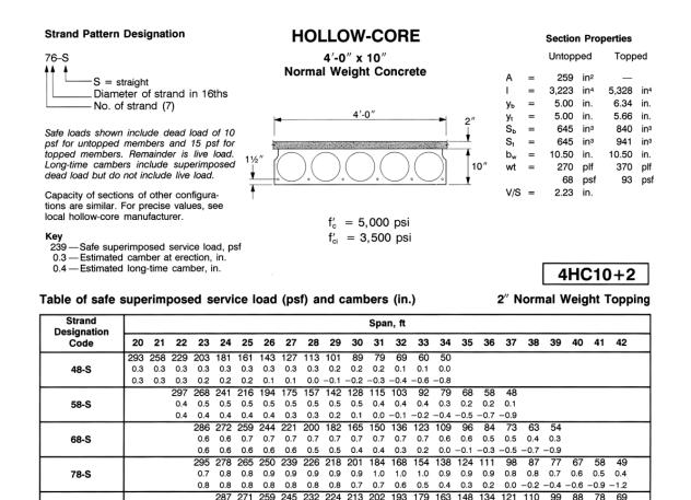
Strength based on strain compatibility; bottom tension limited to  $6\sqrt{f'_c}$ ; see pages 2-2–2-6 for explanation.
