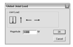
NOTE: <u>Do not</u> put support reactions as applied loads. The analysis will determine the reaction values
