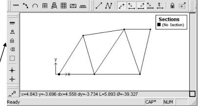
• The support types can be set by selecting the joint (drag) and using the Joint Toolbar (pin shown), or the Frame / Joint Restraint ... menu (right click).
