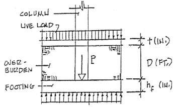
$$q_{net} = q_{allowable} - h_f (\gamma_c - \gamma_s)$$
