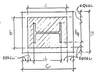
$b = b_f + \frac{(B - b_f)}{2}$  where  $b_f$  is the width of column flange and B is base plate side
