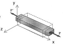
There exists a linear relationship while in the linear-elastic range of the material between *longitudinal strain* and *lateral strain*:
