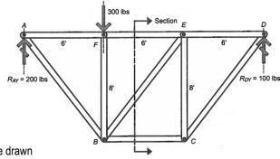
There can be only two intersections when two of the three forces are parallel – at E and B:
