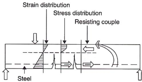
Stresses in the concrete above the neutral axis are compressive and nonlinearly distributed. In the tension zone below the neutral axis, the concrete is assumed to be cracked and the tensile force present to be taken up by reinforcing steel.
