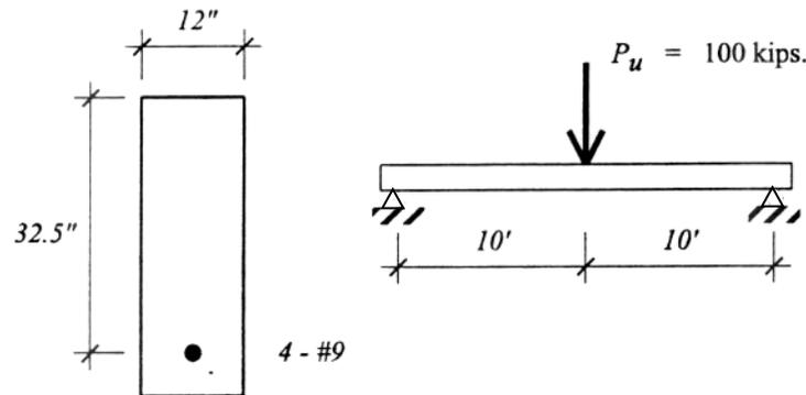
**Figure 5-61:** Simply supported concrete beam for Example 5-15.
