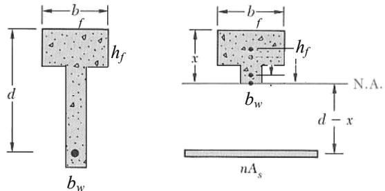
$$b_f h_f \left( x - \frac{h_f}{2} \right) + (x - h_f) b_w \frac{(x - h_f)}{2} - nA_s (d - x) = 0$$
