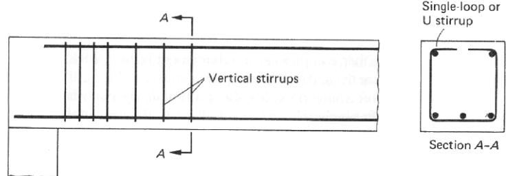
The maximum shear for design,  $V_u$  is the value at a distance of  $d$  from the face of the support.
