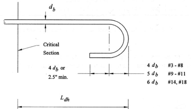
Figure 9-18: Minimum requirements for 180° bar hooks.
