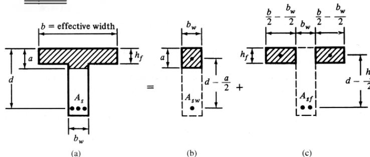
Figure 5.7 Separation of T beam into rectangular parts.
