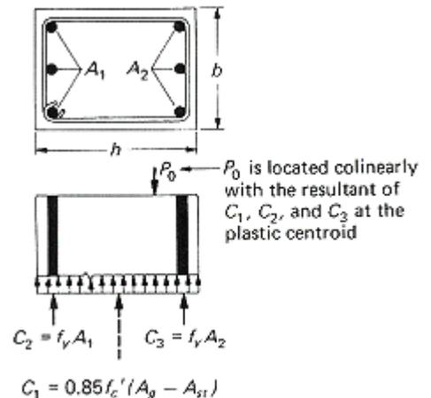
Columns with Bending (Beam-Columns)
