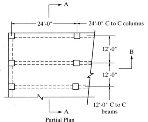
**A. Continuous one-way floor slab**
