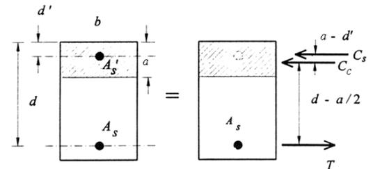
Because the compression steel may not be yielding, the neutral axis  $x$  must be found from the force equilibrium relationships, and the stress can be found based on strain to see if it has yielded.
