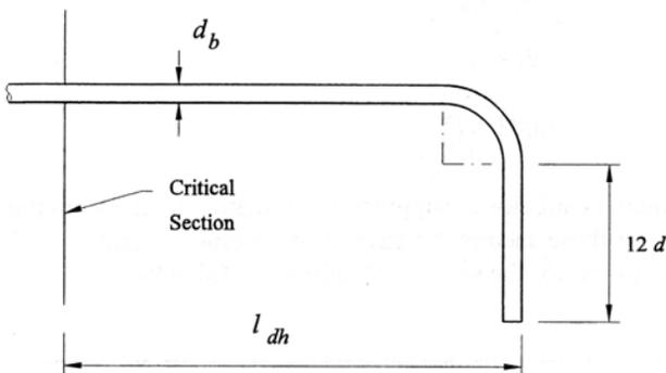
Figure 9-17: Minimum requirements for 90° bar hooks.
