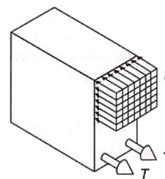
Ultimate strength analysis. (A rectangular stress block is used to idealize the actual stress distribution. Calculations are based on ultimate loads and failure stresses.)
